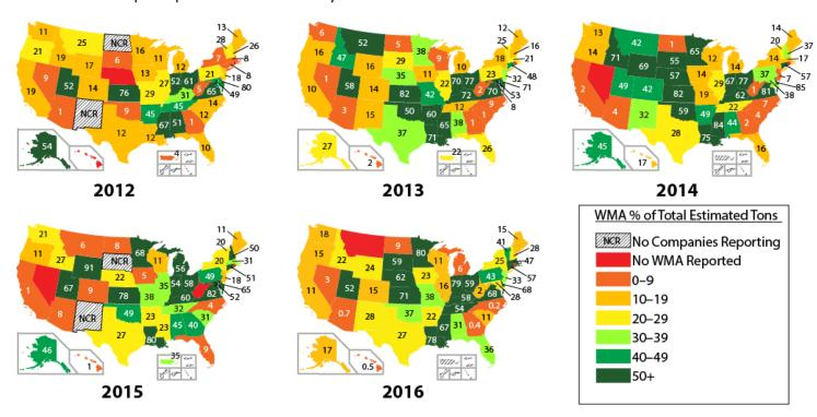
Figure 17: Estimated Percent of Total Production Using WMA by State, 2012–2016
