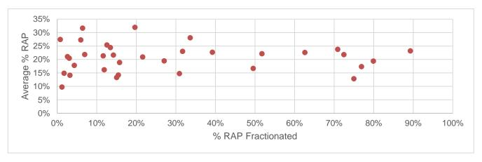
Figure 9: Scatter Plot Showing Reported Average Percentage of RAP in Asphalt Mixtures Relative to Reported Percent of RAP Fractionated, 2016
