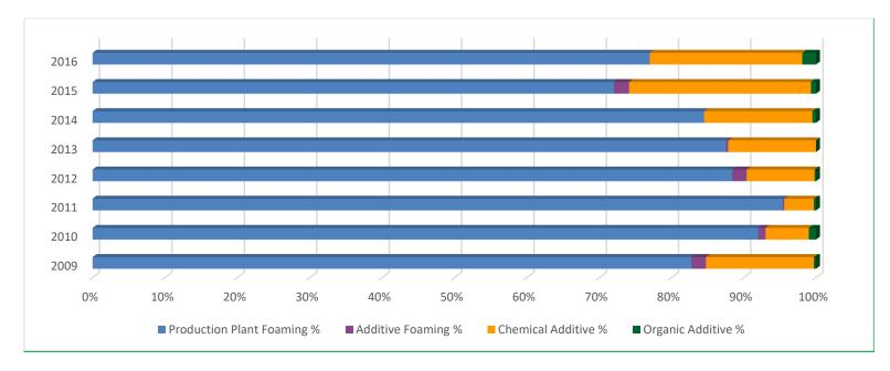
Figure 18: WMA Technologies Used as Percent of WMA Production, 2009–2016
